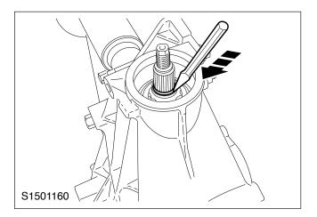
NOTE: Insert a chisel in the circlip groove.11. Unlock the drive pinion nut.
