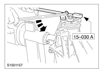
5. Remove the radial oil seals, unlock the bearing housings.
